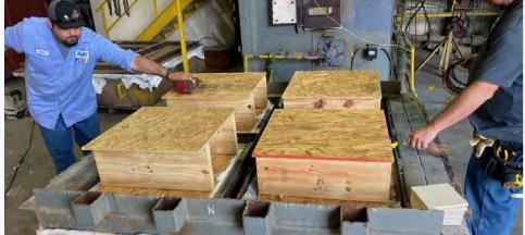
Ceramic coating was used in a floor assembly of OSB achieving a 2-hour rating at a 7 mm thickness.
